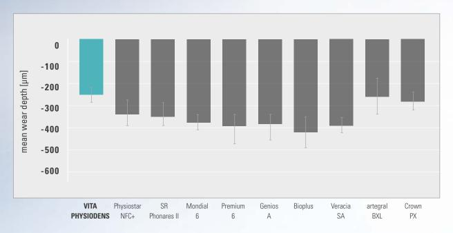
**Graphic:** Average depth of the signs of wear of the abovementioned tooth lines after pin-on-block wear test in the chewing simulator with steatite balls as antagonist and eight test samples each per line.
