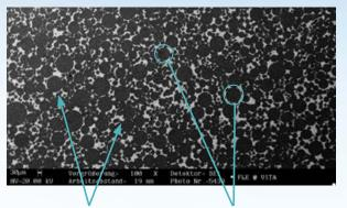
Matrix with polymerized SiO<sub>2</sub>
