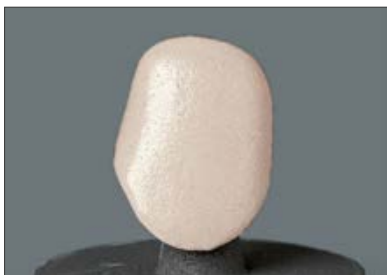
The opaque on a ceramic firing tray shows a light surface glaze after firing.
