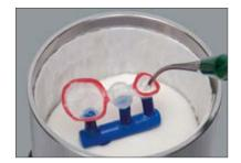
Invest the casting model in accordance with the instructions of the investment material manufacturer and place in the preheating furnace.
