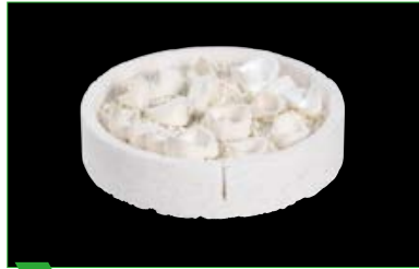
5 Sintering dish MS filled with restorations.
