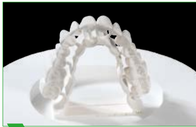
5 Separated and reworked restoration with sintering support.
