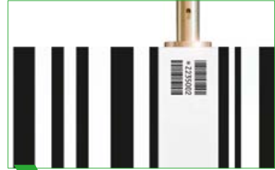
3 Enlargement factor as barcode on block
