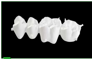
1 Milled restorations immediately after the CAM process.
