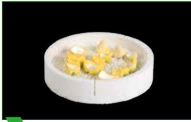
1 Manually pre-colored restorations in the sintering dish MS, ready for speed sintering
