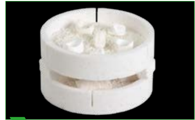
6 Stack sintering of color/multicolor restorations.
