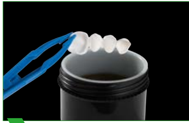
2 Immerse substructure in the coloring liquid with metal-free pincers ...
