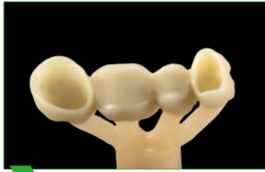
5 Pressed and blasted restoration on the press sprue.
