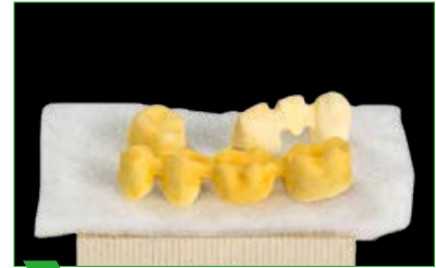
6 Dry the restorations thoroughly before sintering.
