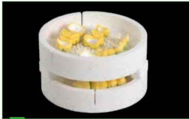
7 Stacks of sintering dishes MS for manually colored restorations.
