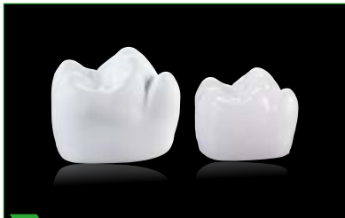
4 Molar before and after sintering; sintering shrinkage of about 20 percent
