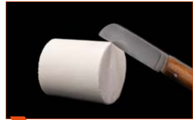
3 Break the edges of the investment ring without allowing investment material to fall into the channel.
