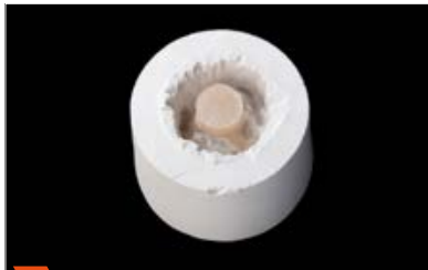
4 Perform rough divestment with Al 2 O 3 (50 µm grain size) at a pressure of 4 bar.
