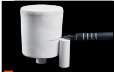
1 Determine the press depth by marking with a second press plunger.
