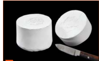
3 Split the investment material carefully using a knife on the predetermined breaking point.
