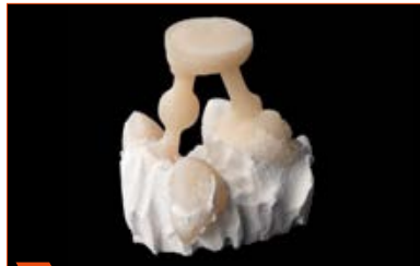
5 Fine divestment and removal of reaction layer at a pressure of 2 bar.
